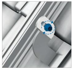
Fasten the connection by tightening the nut (torque of 25 Nm). Make sure that the screw head is first rotated by 90° so that it is anchored in the slot.
