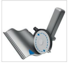
If necessary, remove the interlocking joint at the marked position on the removed tile using an angle grinder (with clay tiles, an expert roofer can use a hammer for this). Remove only the amount of material that is absolutely necessary, work only on the interlocking joint and avoid weakening or damaging of the tile.
